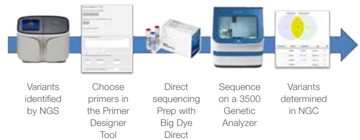
Figure 1. NGS-to-CE workflow. A complete workflow for verifying variants discovered by NGS systems is shown. Applied Biosystems products have been designed to be optimized to work together. NGS variants that are marked for verification can be directly imported into the Primer Designer Tool for picking and ordering appropriate PCR primer pairs that can be directly sequenced with the BigDye™ Direct sequencing kit and the 3500 Genetic Analyzer. The resulting data (.vcf file from NGS and .ab1 trace files from CE) are then aligned and compared in the Next-Generation Confirmation (NGC) tool in Thermo Fisher Cloud.
